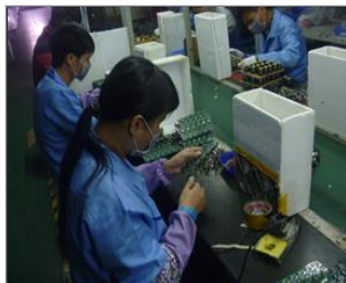
Photo of non-conformity NC-the factory provided active carbon instead of dust-proof mask to soldering worker.JPG
