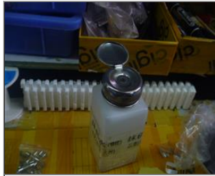
Photo of non-conformity NC-the cleaning solvent at assembly line was not identified with its danger.JPG
